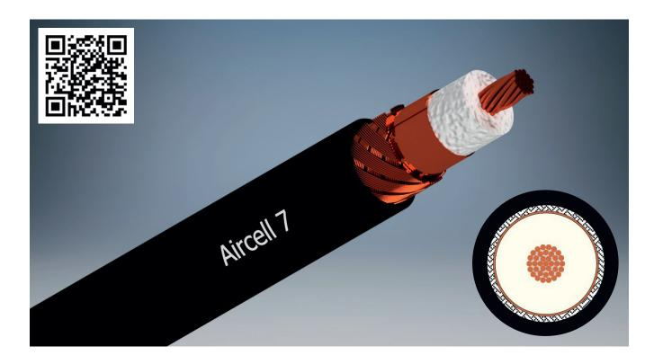
Aircell 7 is an ultraflexible coaxial cable designed for frequencies up to 6 GHz. Due to its low loss in relation to the outer diameter and the small bending radius the cable can be used for numerous RF applications.
