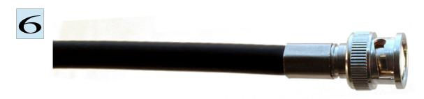
Crimp the crimp jacket with a crimp tool; herewith the copper braid will be trapped between the crimp jacket and the connector housing.
