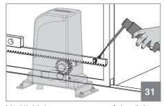
${\bf 03} \bullet {\sf Weld}$  the spacer on top of the pinion.
