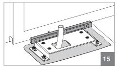
04 • Insert the plate with screws in the concrete while it is still fresh and level it horizontally with a level. Also align it parallel to the gate, keeping a distance of 60mm between them, as visible in picture 16.
