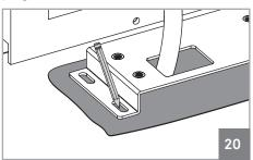
**02** • Mark the place to make the holes for the bushings. Must make the mark at the center of the oval holes of the plate.
