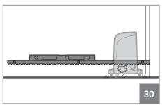
**02** • Place a piece of rack on top of the pinion and level it horizontally with a level.
