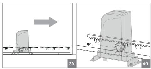
**03** • Close the gate a bit until the other end of the rack rests on top of the pinion and fasten the other support.
