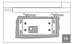
**01** • Place the fixing plate on top of the foundation and align it parallel to the gate, keeping a distance of 60mm between them, as visible in Figure 19.
