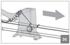
**07** • Remove the piece of auxiliary rack and open the gate until the other end of the rack stands on top of the pinion. Weld the spacer.
