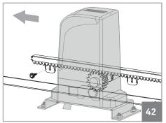
**05** • Open the gate until the other end of the new rack is on top of the pinion rack and fasten it to the gate.
