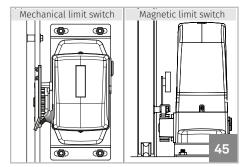
01 • Place the opening limit-switch plate in the rack so that it can trigger the limitswitch of the motor before the gate gets to opening stopper. The mechanical limit switch is activated when the plate is in contact with the spring. The magnetic limit switch is activated when the magnet is aligned with the motor reader (Fig. 45).
