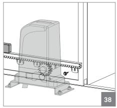
**02** • Fasten the support of the rack over the pinion to the gate.
