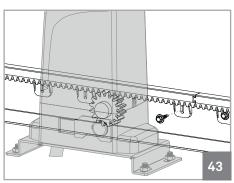
**06** • Open the gate until the other end of the rack stands on top of the pinion. Fasten it to the gate.
