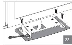
**04** • Place the fixing plate on the foundation in cement respecting the distances of image 19. Use a level to levelit horizontally and fasten it with M10 screws.
