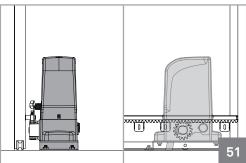
•Check that the distance between rack and motor remains unchanged and this engages the teeth of the pinion of the engine correctly (over time can happen some distortion).
