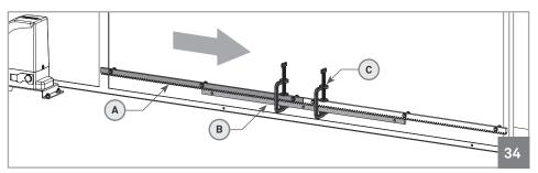
**05** • Close the gate a bit, so that the rack is not being supported on the pinion anymore and apply another piece of rack (A). To synchronize the teeth with the piece already installed, use an additional piece of rack (B) and place it under the union of the other two, holding them with clamps (C).
