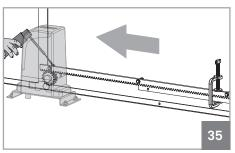
**06** • Open the gate to support the point of the new piece of rack on top of the pinion and weld the spacer.
