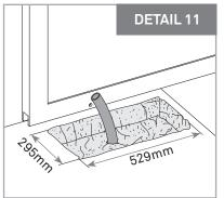
01 • Make a hole in the ground to create a foundation in concrete. The dimensions shown are these recommended to create the foundation. You must leave tubes in the middle of the hole for the passage of cables for power and accessories, as shown in the detail of image 11.
