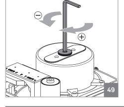
The tuning must achieve a balance between the gate's irreversibility and the engines power.
