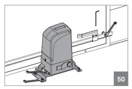
• Check all screws of the automation such as the fixing plate to the ground, the plates of the limit switches, motor and the gear rack.
