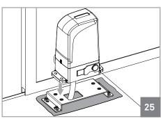
**02** • Place the motor in the fixing plate.
