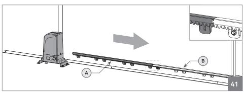
**04** • Close the gate a bit, so that the rack is not being supported on the pinion anymore and apply another piece of rack (**A**), fitting it into the rack already installed (**B**), as you can see in detail of image 41.
