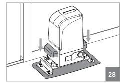
**05** • Reassemble the motor's side covers to hide the screws.
