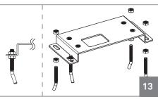
03 • Attach the screws to the plate with nut and counter nut as shown in picture 13.
