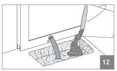
02 • Fill the hole with fresh concrete and smooth the top part where you will fix the plate.
