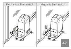
03 • Move the gate to the closed position and repeat steps 1 and 2 to fix the closing limit-switch plate to the rack.
