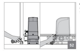
•Lubricate all systems/axis of movement of the gate. Lightly lubricate with spray the rack and pinion.
