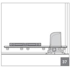
**01** • Place a piece of rack on top of the pinion and level it horizontally with a level.
